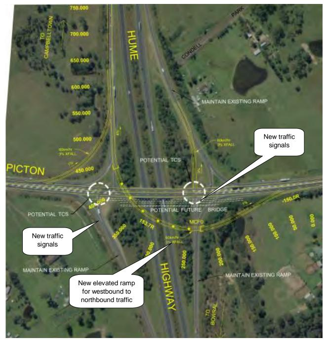
Figure 5.9 Proposed Hume Highway/Picton Road interchange upgrade
